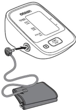
The blue plug at the end of the air tube attached to the cuff should be inserted into the side of the blood pressure monitor.
